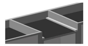
4. Test fit the sink in the opening that was created in the previous steps. The entire weight of the sink should be supported by the support frame. Verify that the sink is in line and level with the top of the cabinet.
