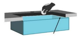
6. Allow the silicone to dry for 24 hours. Then install your drain, faucet, and other accessories according to the installation instructions.
