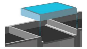
5. Set the sink in place and fill in any gaps below the sink front and between the sink and countertop with silicone sealant. Hold the sink in place to secure. Place the countertop onto the sink and remove any excess sealant from all surfaces.
